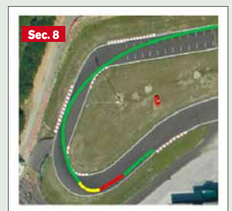
Sector 8: Brakes on for the last time before returning to the finish line. In this case, it is advisable to brake as much as possible and then cut on the curb inside and speed up again all the way to the finish line.
